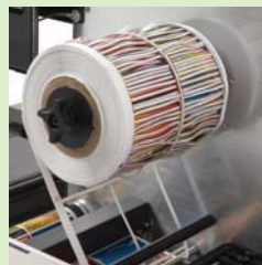
Removal of waste matrix
